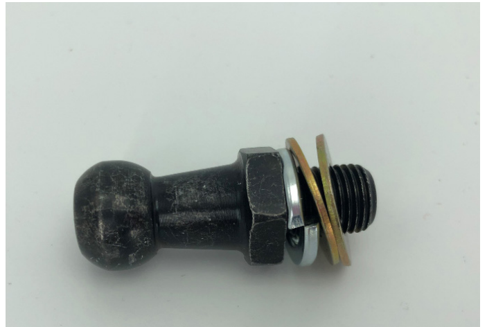
Washer orientation on Pivot Ball
